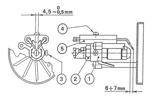
**Please note**: To set the system to stop the baffle plate (1), loosen the screw (3). To set the electrode system, loosen the screw (4).
